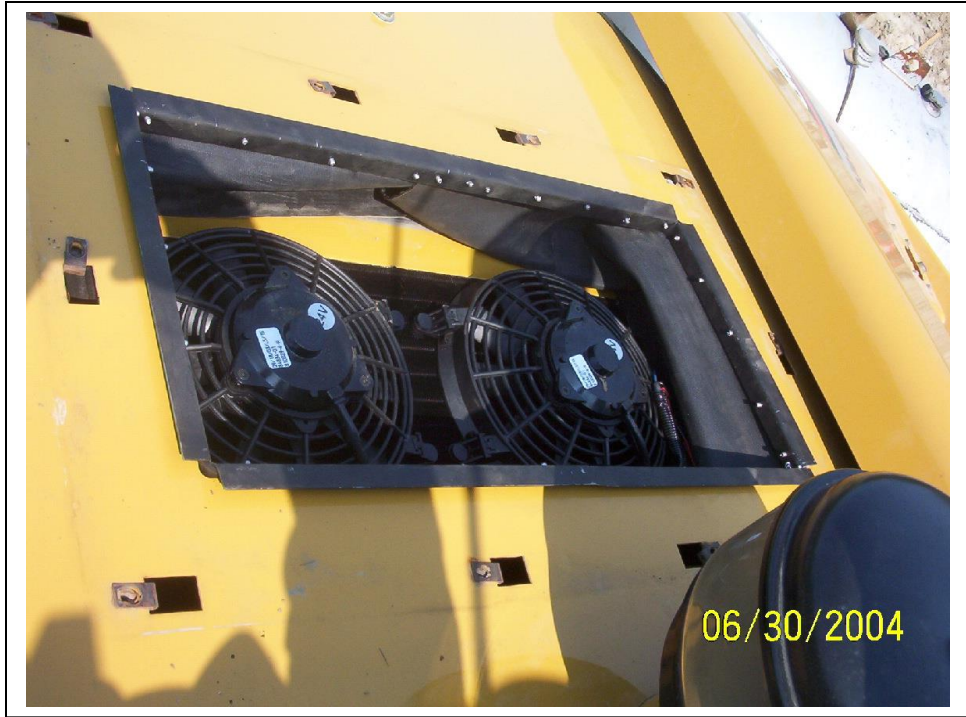
Condenser mounted in place showing the condenser fans.
