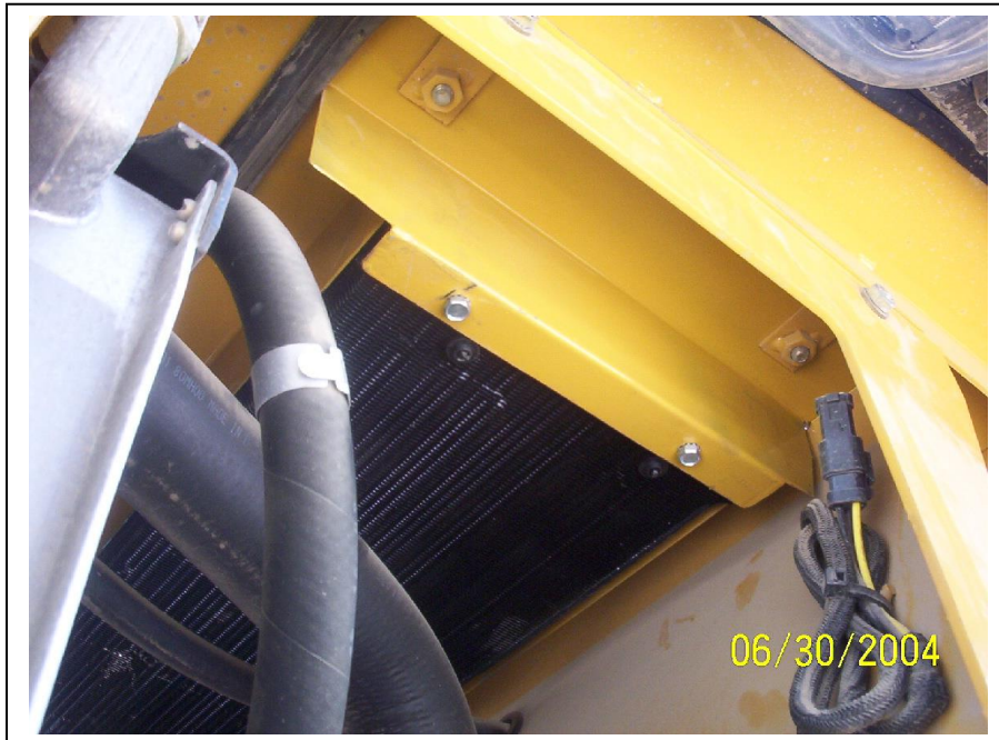
Left side of condenser mounted in place.
