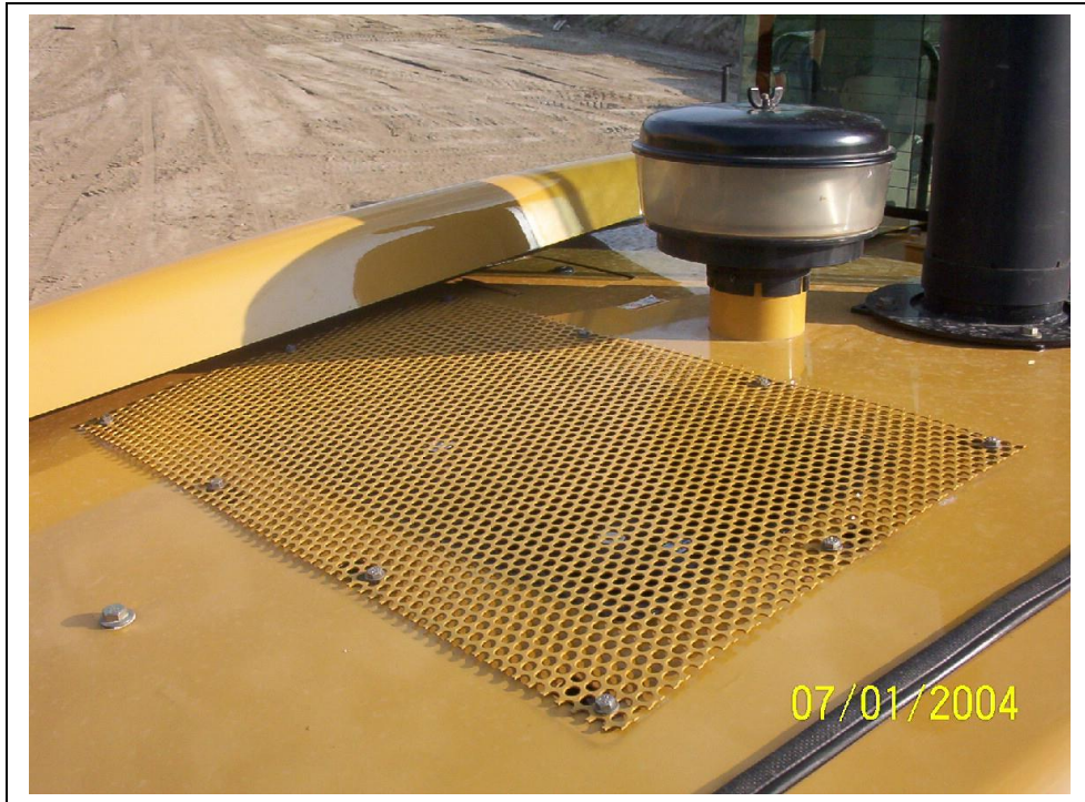
New cover (supplied) over the condenser.
